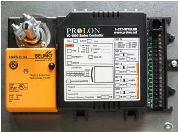
Figure 3. PL-VC1000 VAV Zone Controller
