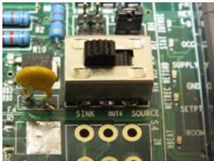
Figure 5. Dry contact output PASSIVE ('SINK')
