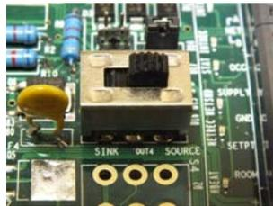
Figure 6. 24Vac output ACTIVE ('SOURCE')
